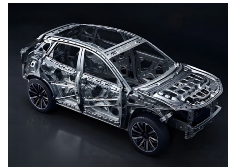
SAFE BODY STRUCTURE 85% HIGH-STRENGTH STEEL
