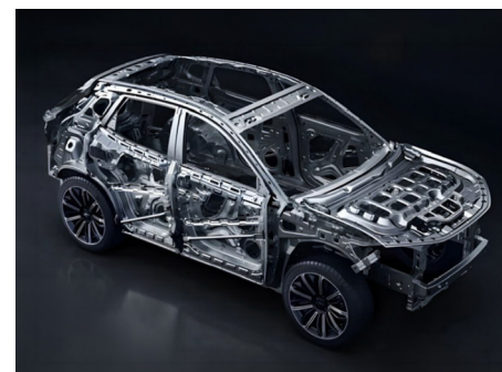
SAFE BODY STRUCTURE 85% HIGH-STRENGTH STEEL
